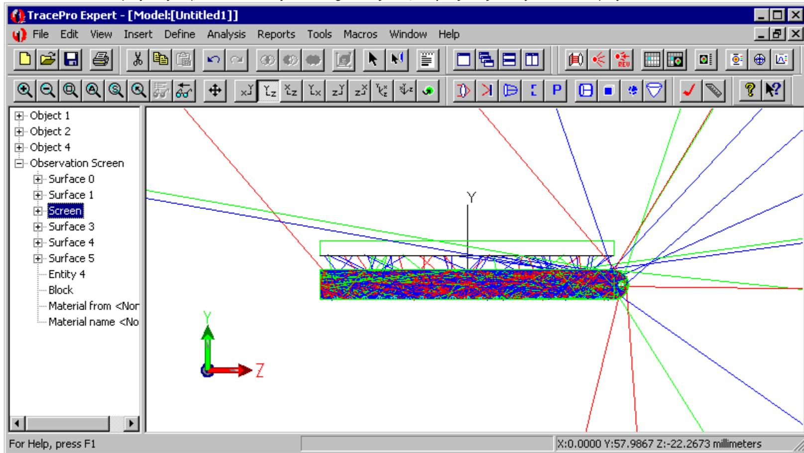
The observation screen was set to be completely absorbing and most rays reach, and stop at, its bottom surface. Rays missing this object are shown bypassing it. The color of each ray indicates its flux. Red rays have flux from 100 to 66 percent of their beginning ray flux. Green rays are between 66 and 33 percent and blue rays are between 33 and 0 percent.
