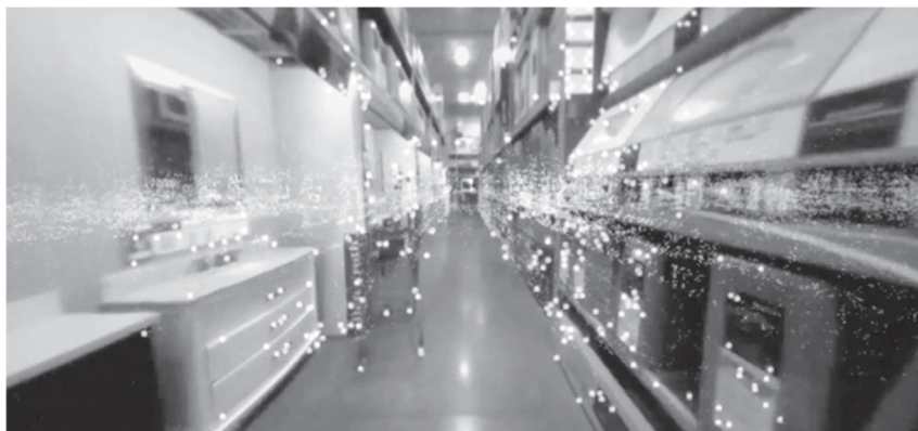
Figure 22.6 Typical SLAM data cloud from ARCore.
