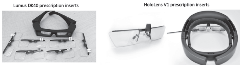
Figure 21.3 Examples of ophthalmic lens inserts for single far-field vision correction in AR and see-through MR headsets.
