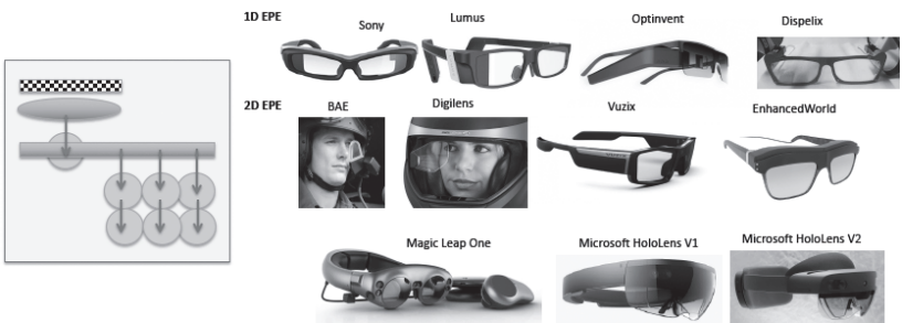
Figure 8.5 Waveguide-based exit pupil replication in 1D (top) and 2D (center and bottom).
