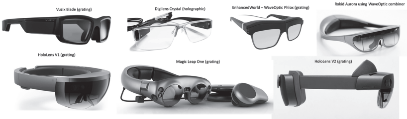
Figure 14.8 Smart glasses and AR headsets that use 2D EPE diffractive or holographic waveguide combiners.
