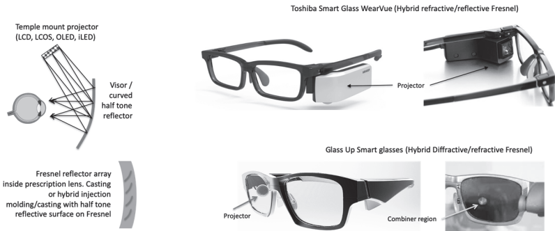
Figure 11.10 (upper) Hybrid refractive Fresnel combiner (Toshiba) and (lower) hybrid diffractive Fresnel (Glass-Up).
