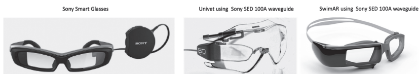
Figure 14.6 Sony Smart Glasses and third-party versions using a Sony SED100A waveguide combiner.
