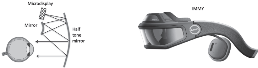
Figure 11.9 Off-axis multiple reflector architecture (IMMY, Inc.).
