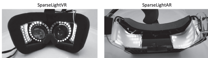
Figure 20.3 Peripheral display using individual LED arrays (Microsoft Research 2016).
