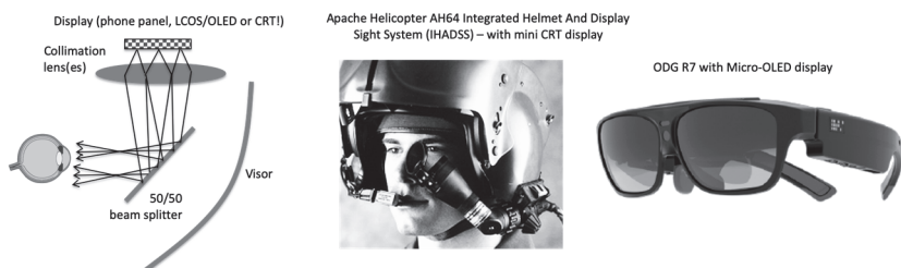
Figure 11.1 Tilted half-tone mirror combiner architectures (IHADSS and ODG R7).
