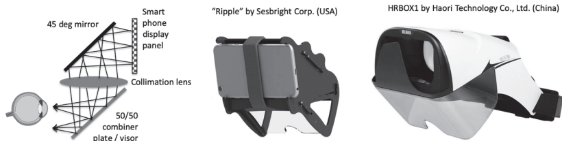
Figure 11.2 Vertically positioned smartphone display with flat half-tone, low-cost AR combiner architectures.
