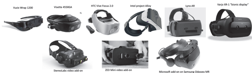
Figure 10.1 Video see-through headsets, either fully integrated (top) or as aftermarket stereo-camera add-ons (bottom).
